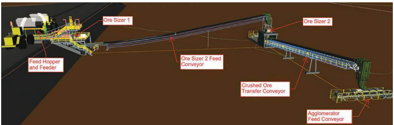
Figure 8: Run of Mine (ROM) and crushing circuit diagram
